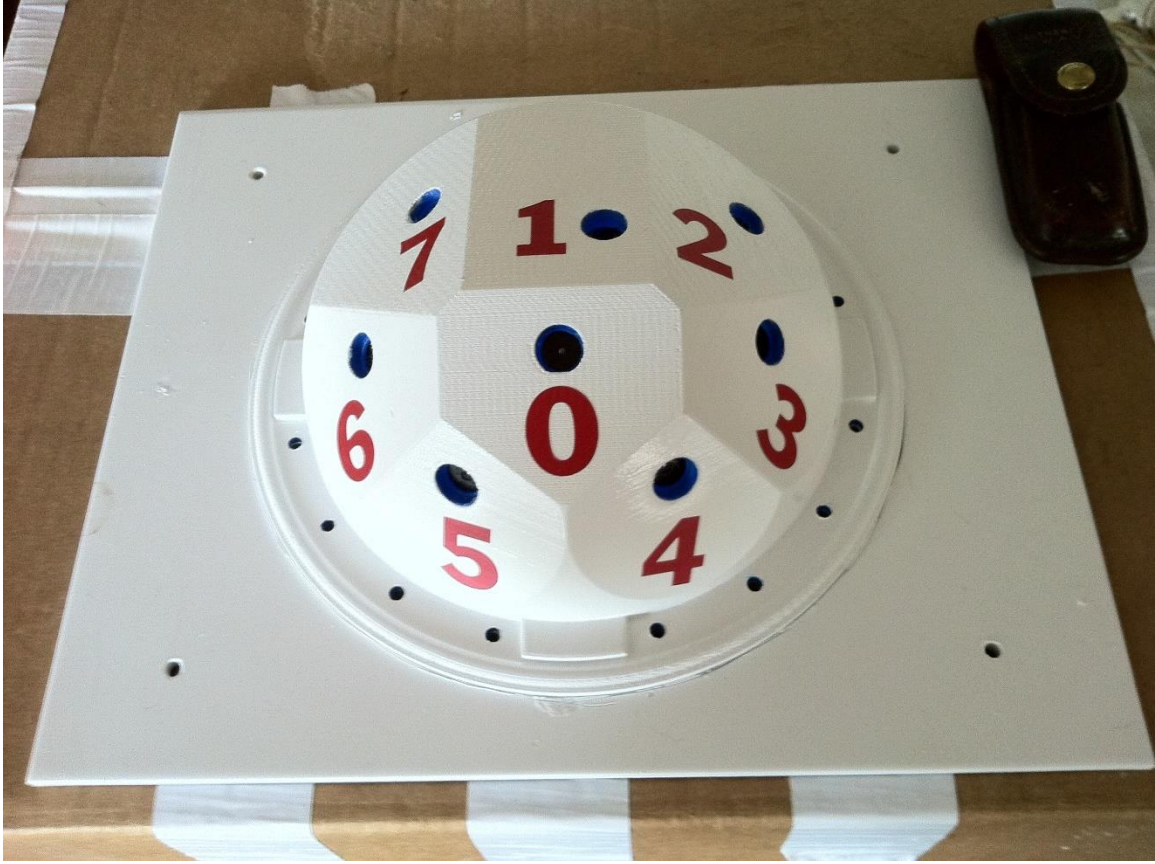
Figure 5-20. Outer shell location and labeling of all eight views in three equatorial planes labeled L0 through L7.
