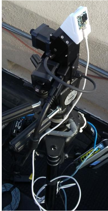
Figure 5-11. Stationary FLIR Lepton with breakout on tripod.
