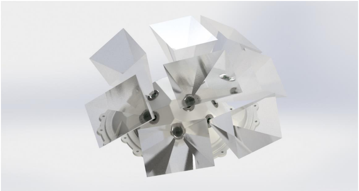
Figure 5-24. Rendered Ladybug Version 2 view of the apparatus with the views emerging from the individual windows shown as transparent glass.
