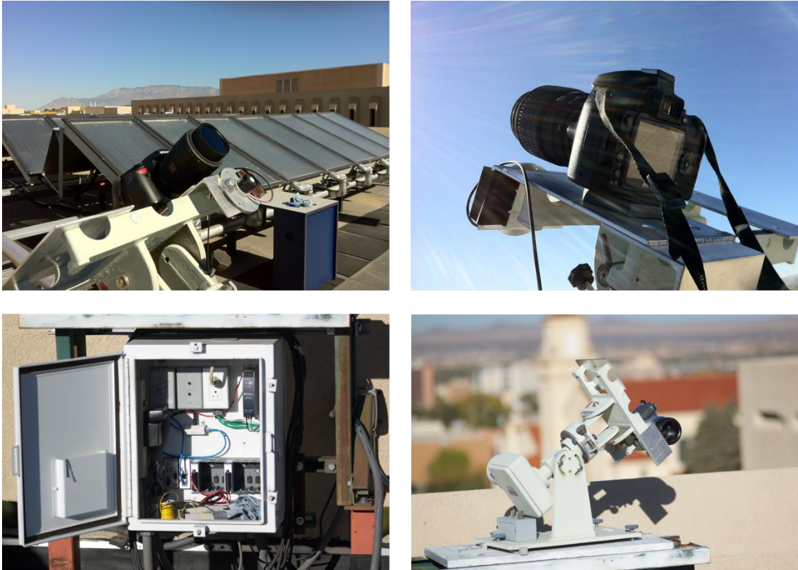
Figure 5-4. A. Top Left/Right; Nikon D40 charged coupled device camera utilizing a 950 nm long pass filter. Facing directly at the sun, is a LI-200R Pyranometer for irradiance measurements. B. Bottom right; shows an Eppley Laboratory solar tracker to track the sun. C. Bottom left, shows UNMs National Instruments NI-CompactDAQ chassis activation system to automatically take pictures of the sun and irradiance measurements at the same time at 10 second intervals.
