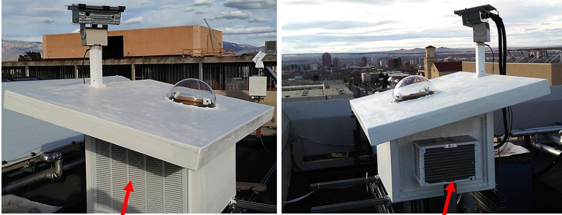
Airflow vents keep the air conditioner from cycling too often.
