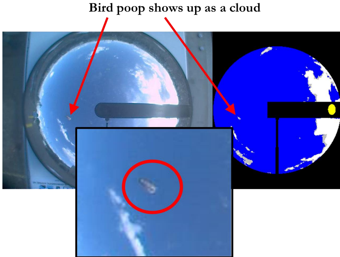
Figure 3-11. Total Sky Imager (TSI) pictures from Sandia National Laboratories. The picture on the right is the automated cloud detection algorithm built into the TSI system. The bottom TSI also mistakes the bird poop as a cloud.
