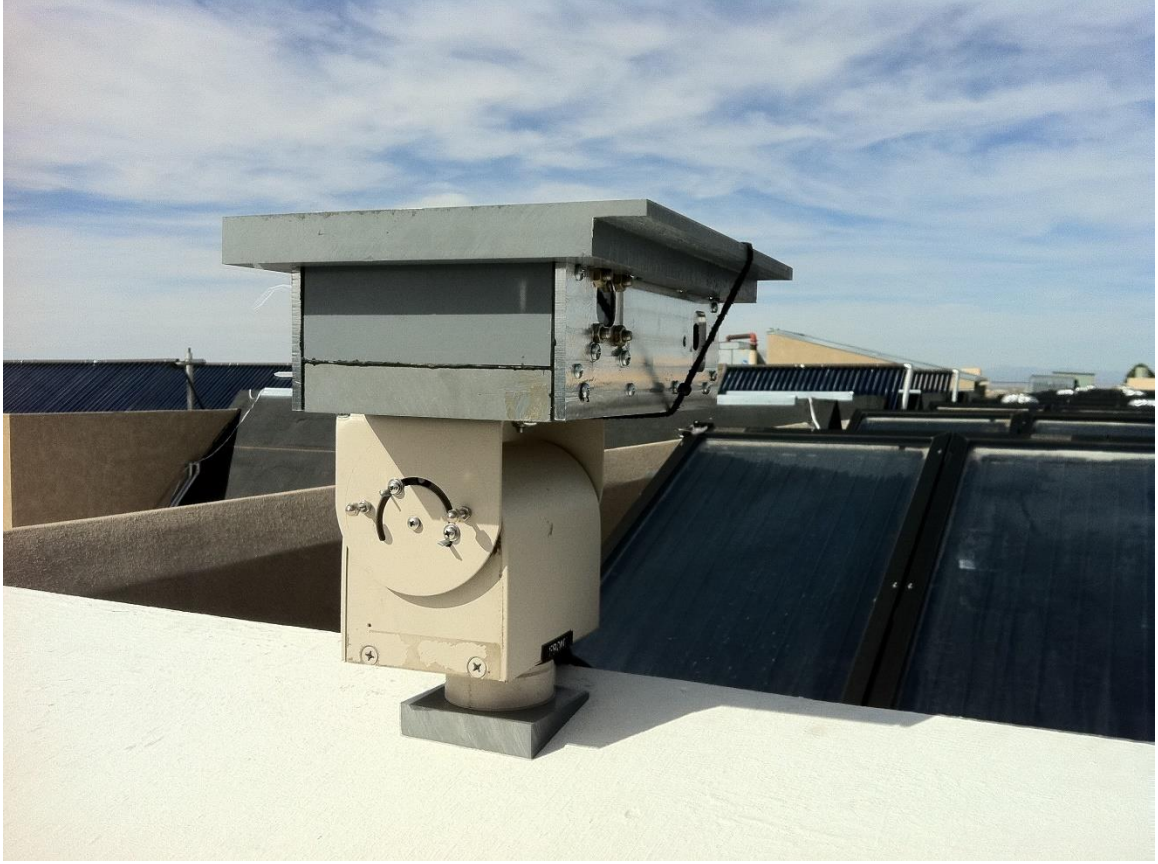
Figure 5-17. Camera Box containing the far and near-IR cameras. The apparatus uses a Pelco PT280 pan tilt unit with cylindrical coordinates. The internal components are shown in Figure 5-18 below.
